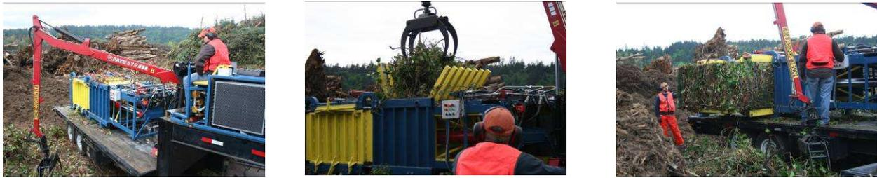
**Figures 3.** Field trial of prototype biomass baler at BRC Inc. yard waste facility in Auburn, WA.
