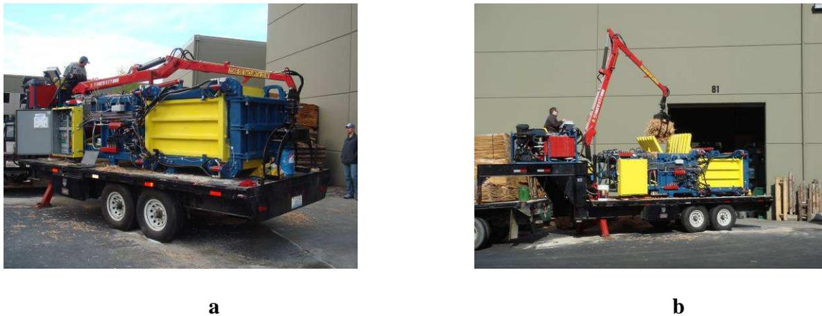
**Figures 2a, 2b.** Fully assembled self-loader trailer with prototype baler and grapple during initial testing in April 2008.
