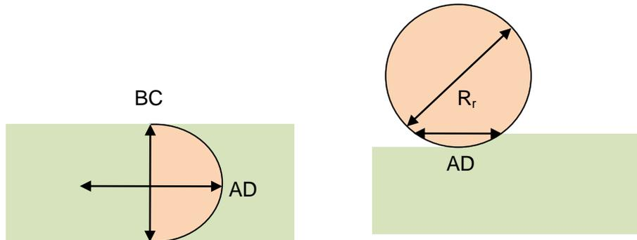
**Figure 8.** Schematic of plan view of elliptical contact area between large diameter roller and round wood log showing the length of the contact ellipse (AD) and width (BC).
