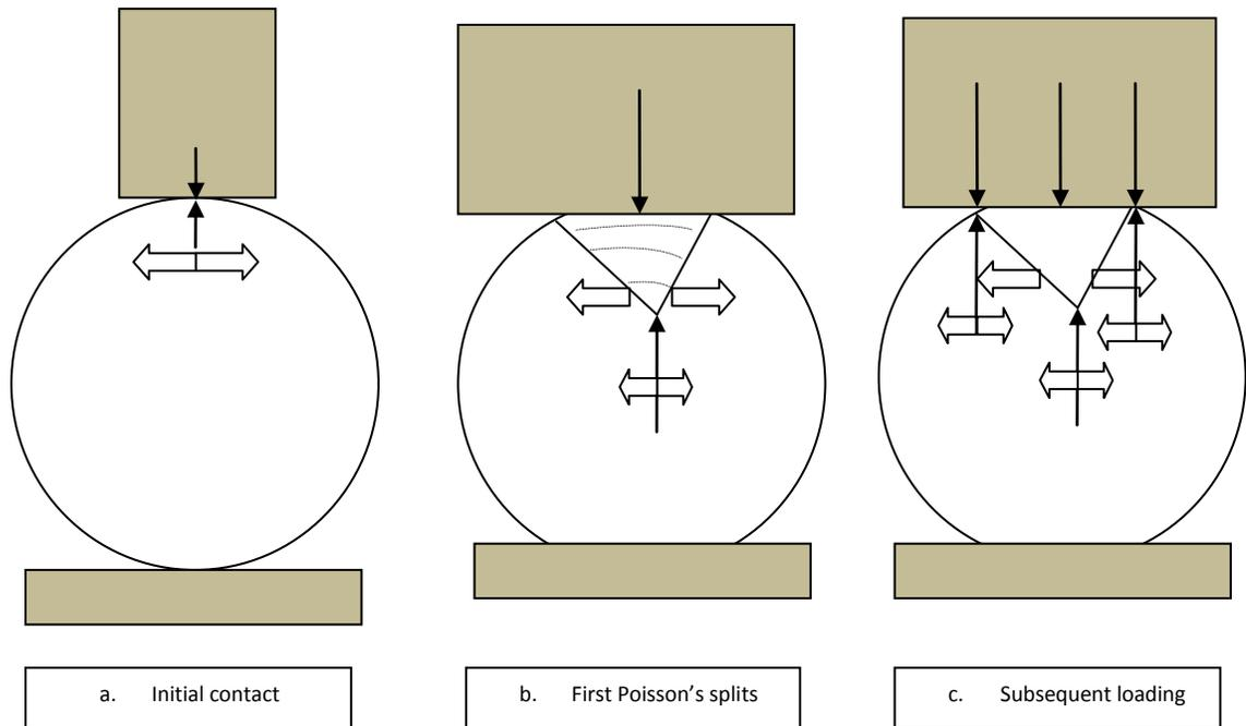
**Figure 4.** Depiction of the stages of failure for a round wood pole section subjected to compression.
