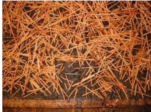
Figure 2. A “high storage” 2002 prototype blend of engineered wood-strand material at 70% soil cover.
