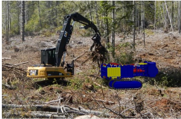
Figure 3. Overlay of conceptual track-mounted self-propelled baler on a logging site with an actual forest woody biomass loader. The baler is approximately to scale with the loader.
