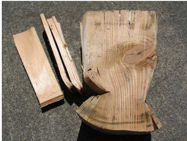
Figure 10 Here it can be seen that there is significant compression failure in the region near the blade and wherever there is a force applied to resist the block movement.
