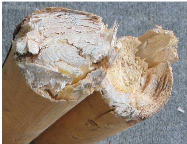
Figure 8: Catastrophic failure from parallel to grain tension, not shear.
