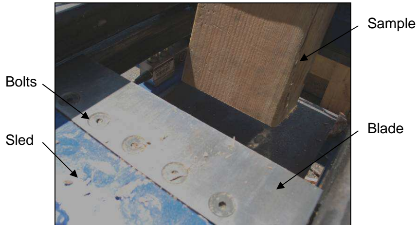
Figure 2: Shear blade attachment
