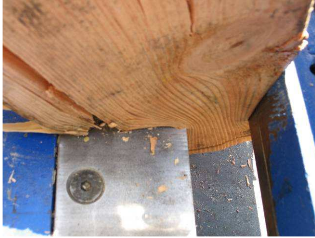
Figure 9: The blade starts to cut by causing local compression failure.
